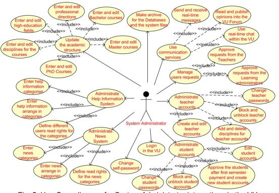
Fig. 5. Use-Case diagram for System Administrator interactions in the VU
