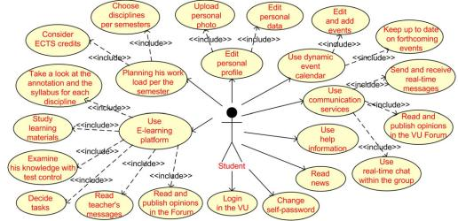
Fig. 3. Use-Case diagram for Student interactions in the VU
