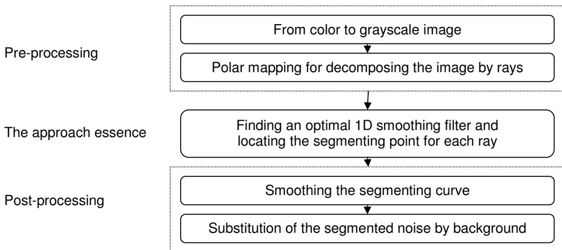
Fig.1. Stages of the image processing for artifact-noise isolation
