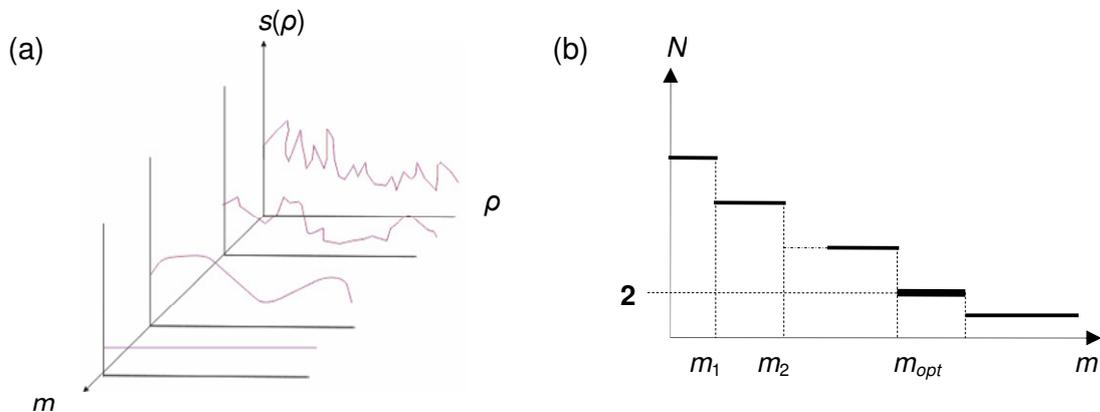
Fig.3. Illustration of the monotonicity of  $N$  (number of maxima) on the smoothing level  $m$  (filter width): (a) the signal  $s = s(\rho)$  after smoothing with increasing  $m$ , and (b) an optimal value  $m_{opt}$  exists for  $m$ ,  $m \geq 1$ .
