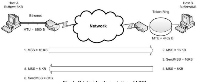
Fig. 1. Original Implementation of MSS
