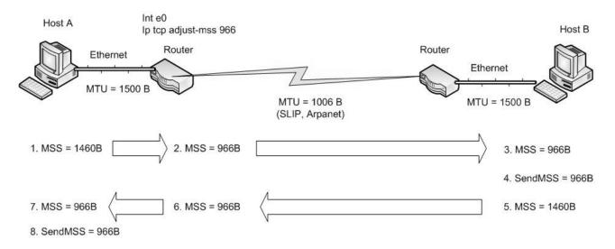
Fig. 3. Router assisted avoiding of fragmentation
