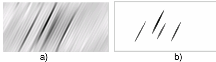
Fig. 5. a) Inverse FT alongside the slope, b) Extraction of the black lines
