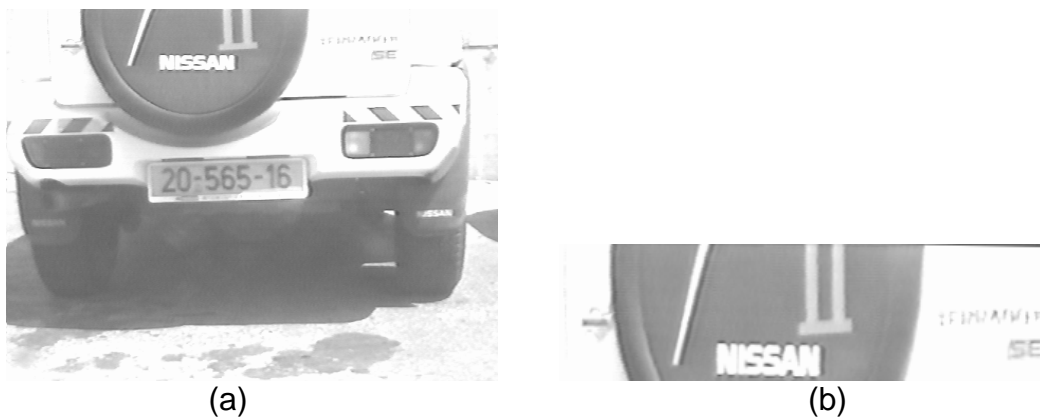
Fig.4. A regular and a reverse intensity situation: (a) a source image; (b) wrong plate candidate with dominating dark levels.
