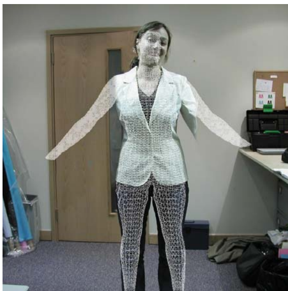
Figure 1 3D scan superimposed on the photograph to approximate camera Natural Global Illumination
