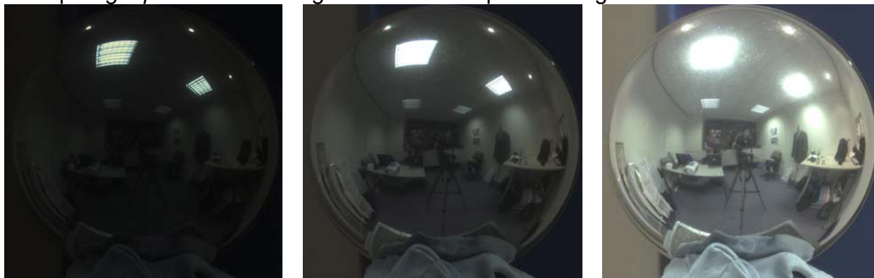
Figure 2 Light probe Radiance measurement of our designer's room the images depict the HDR light probe as 3 low dynamic range images at different f-stops.
